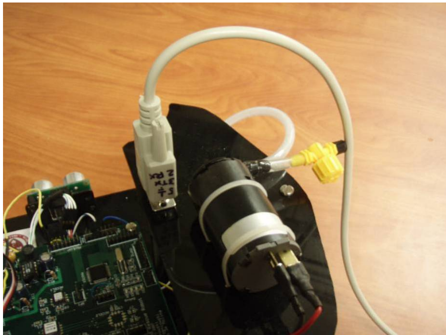
Figure 36: Serial Cable connected to Debug Port
